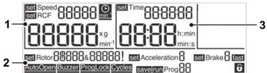
Fig. 9: Display of the "Spincontrol L" control system
