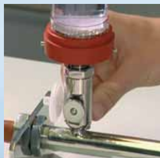
2 | Apply vacuum and filter the sample
