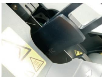
2. Push the blade remover tool over the blade.
