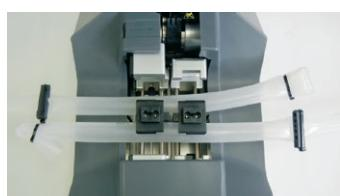
3. Insert the tubes into the tube holder and close cover.
