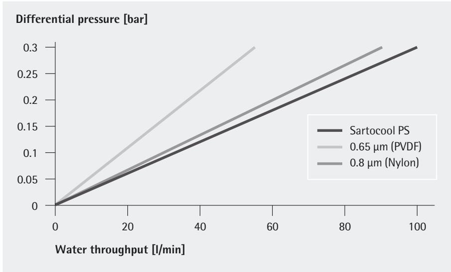
**Stability: Reduction in Flow Rate after 20 Steam-Sterilization Cycles, 134°C, 30 min**
