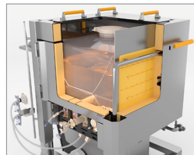
Heat exchange jacket and temperature control
