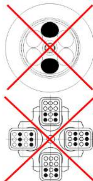
Fig. 9: Permissible and impermissible loading of an angle rotor and a swing-out rotor (example illustrations)
