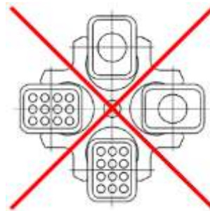
Fig. 8: Permissible and impermissible loading of the swing-out rotor with different tube sizes (example illustration)
