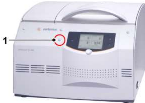
Fig. 30: Position of the opening for the emergency lid release
