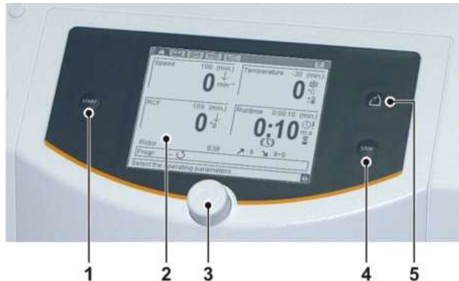
Fig. 10: User interface of the Spincontrol S control system
