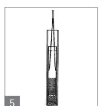
5. Or remove the floater with opened forceps to have access to the concentrate (Fig. 5).
