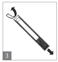
3. Centrifuge in a laboratory centrifuge accepting up to 17×100 mm tubes (Fig. 3). Maximum relative centrifugal force: 2,500 g with swing head rotors, 2,000 g with angular head rotors (see graph). When filtering concentrated protein solutions, for example serum or blood, start with 5 minutes centrifugation at half of the maximum rpm. When filtering solutions containing lipids such as milk, only use an angular head rotor.
