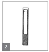
2. Re-insert the floater, membrane side down, and let it slide down onto the surface of the sample. Allow the centrifuge tube to stand (Fig. 2) for approx. 5 minutes to ensure complete wetting of the membrane. Exception: to filter noncoagulated blood, precentrifuge the tube for about 2 min. before inserting floater in order to avoid hemolysis. Do not re-insert closing cap for centrifugation.
