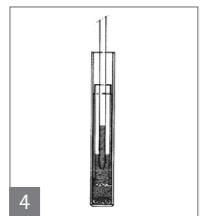
4. Pipet out the filtrate (Fig. 4) as soon as possible after completion of centrifugation (filtrate will slowly diffuse back into the concentrate).
