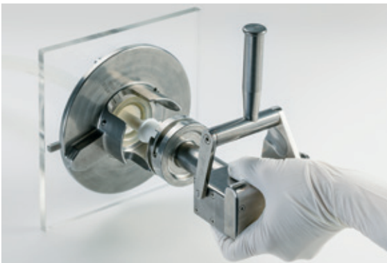
Port rotated and being opened
