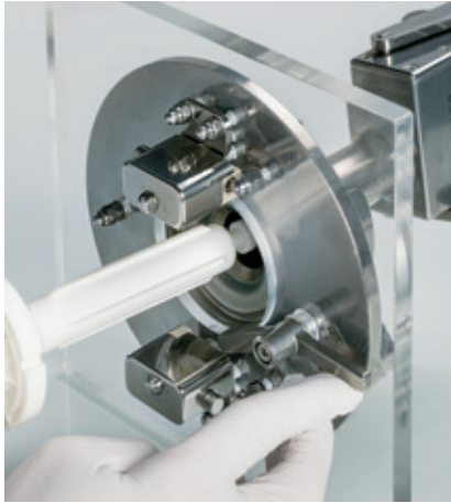
Interlock lifted during connector device insertion
