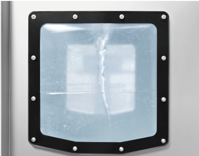
Fig. 8: Vortex at 475 rpm in a 200 L Flexsafe® Bag for Pro Mixer
