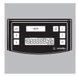
A self-test runs automatically, at the end of which the readout shows **0.0** q.
