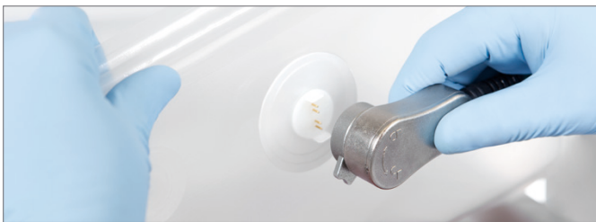
Figure 1: Viable biomass sensor (BioPAT® ViaMass) integrated in the Flexsafe® RM bag – connection to the hardware component.
