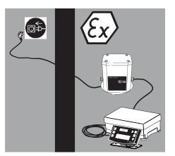
In order to connect the equipment to the power supply, use a correctly installed wall outlet with a protective grounding conductor (PE) and a fuse of a maximum 16 A.
