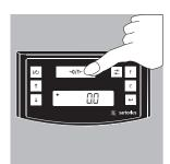
If a different value is displayed: Tare the scale using the 90% key (Zero/Tare).
