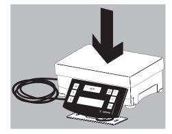
Place the weighing pan on the balance.
