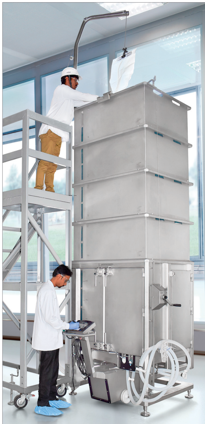
Mixing trial performed at 3000L scale
