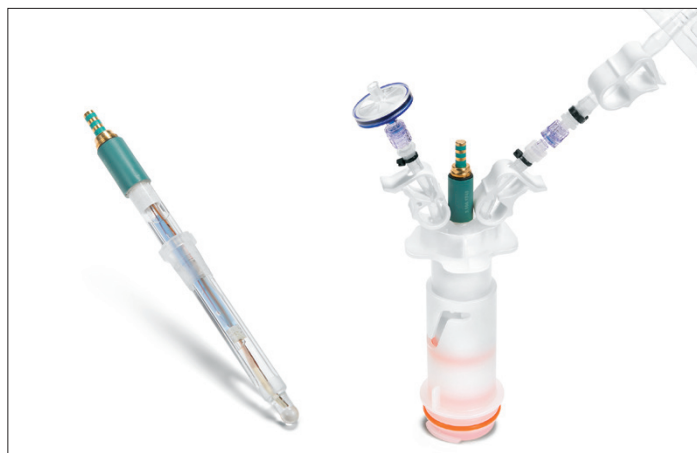
Picture: pH electrode and pH sensor
